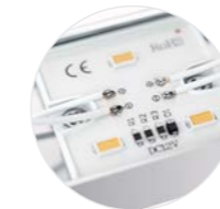
LED modules Bright LED backlighting with modules 5730 and IP67 ingress protection standard
